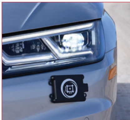
▲ Fig. 2 EAGLE radar attached to the front car bumper.
