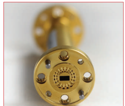
▲ Fig. 4 To prevent damage to the pin surfaces, the front face of the CWF has an outer rim 3 mils thicker than the pin array.
